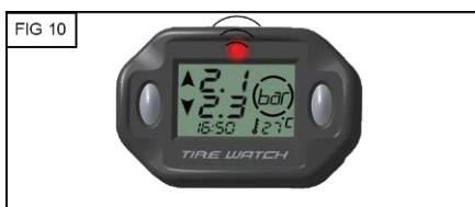
FIG 10 – PRESSURE THRESHOLD CROSSING ALERT
