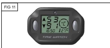
FIG 11 – TEMPERATURE THRESHOLD CROSSING ALERT
