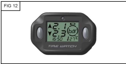
FIG 12 – LOW BATTERY DISPLAY ALERT
